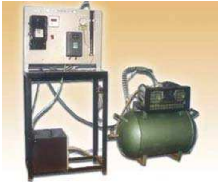
Measuring efficiency of compressor.
